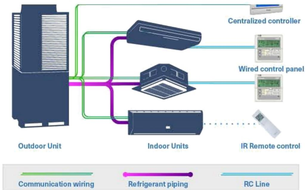
Communication wiring consists of a 2 wired cable, chained from the outdoor to all indoors, creating an internal closed loop network, that is an essential part of any VRF installation.
